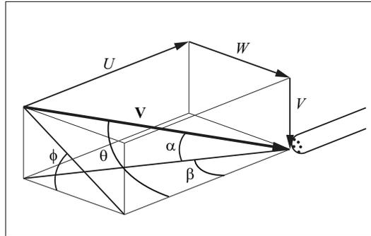
Figure 4: Graphical representation of velocities in pitch/yaw and spherical coordinate systems.
