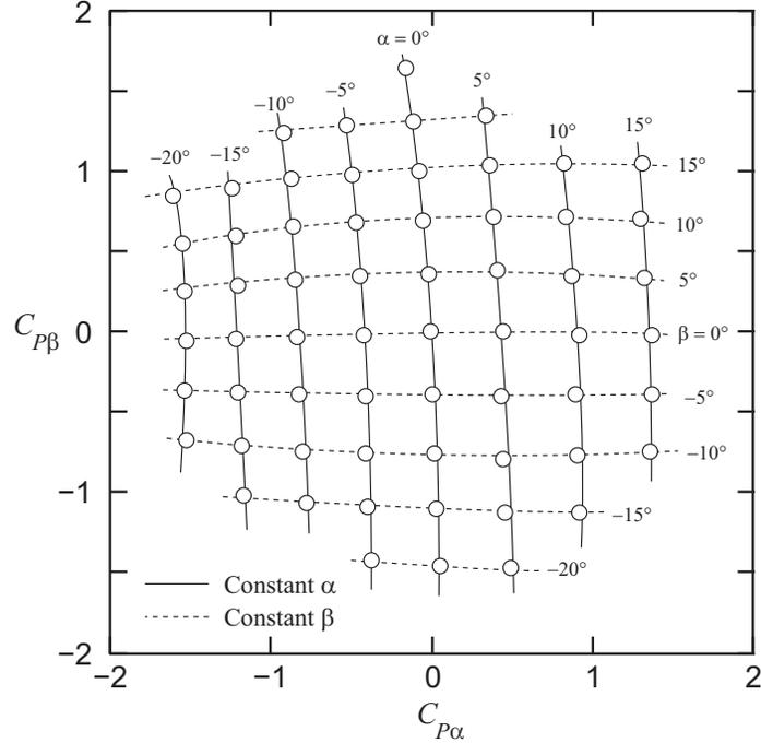
Figure 3: Coefficients of pitch and yaw for a seven-hole probe at small angles.
