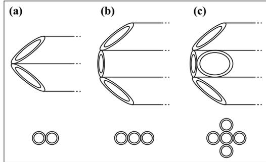
Figure 1: Geometry of common multi-hole pressure probes. (a), Two-hole yaw probe; (b) three-hole yaw-stagnation probe; (c), five-hole cruciform probe.
