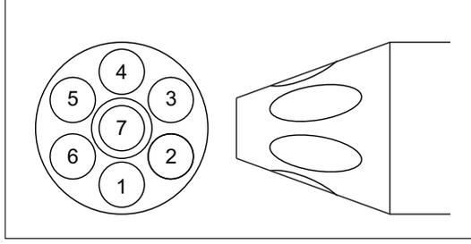
Figure 2: Typical geometry and hole numbering convention for a seven-hole pressure probe.
