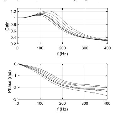
Uncorrected and corrected measurements, 800 Hz, white noise input at ±PFS
